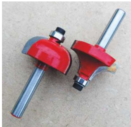
▲ Pic.8 Matching router cutters for flaps and centre piece
